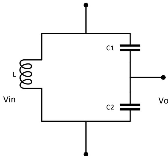
**Figure 4: Capacitance Voltage Divider.**
