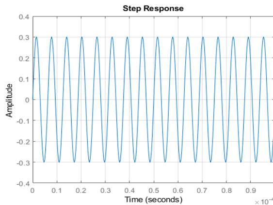
**Figure 6: Undamped Harmonic Oscillations.**
